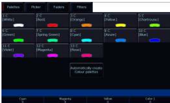
“Colour Palettes” window after “Automatically create colour palettes” has been selected with colour mixing fixtures patched.
