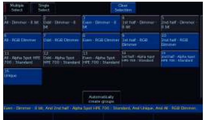
Groups window with various fixtures current selected highlighted in blue
