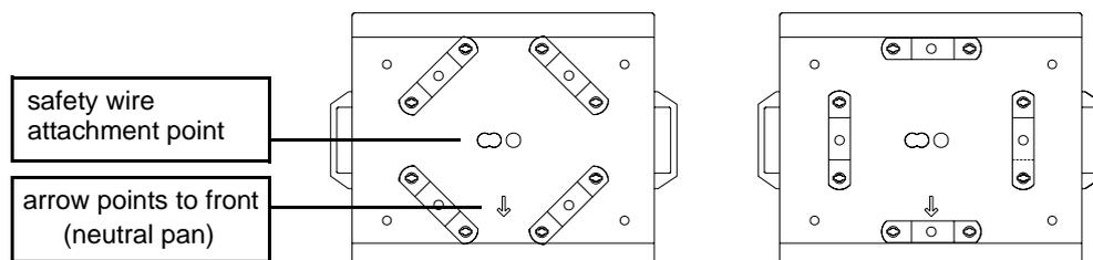
1. Verify that the rigging clamps (not included) are undamaged and can bear at least 10 times the weight of the fixture. Bolt the clamps securely to the clamp brackets with a grade 8.8 (minimum) M12 bolt and lock nut, or as recommended by the clamp manufacturer.
